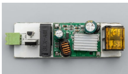
Figure 14: Overvoltage Protection Board.
