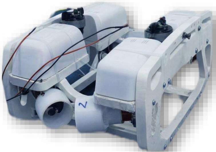
Fig. 4: Titamarine Initial Chassis Frame Fully Assembled
