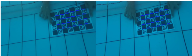
Figure 18 : Stereo Calibration Marker Detection
