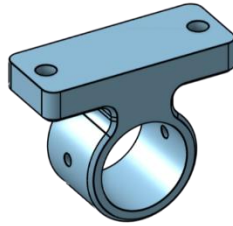
Figure 10 Fisheye Camera Bracket (3d printed)
