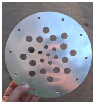
Figure 12: Custom laser-machined rear aluminum face.
