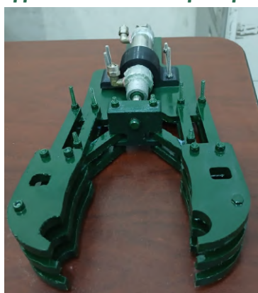
Figure 25: Photograph of the custom- machined HDPE Grippers.
