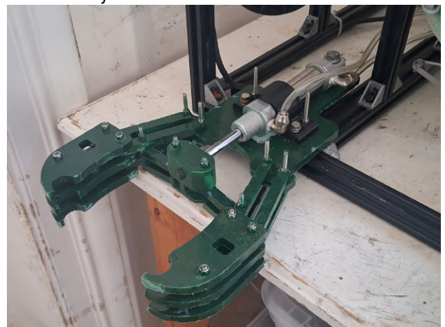
Figure 14: Leviathon's gripper in open position.
