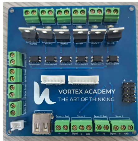
Figure 16: Leviathon's custom main control PCB.
