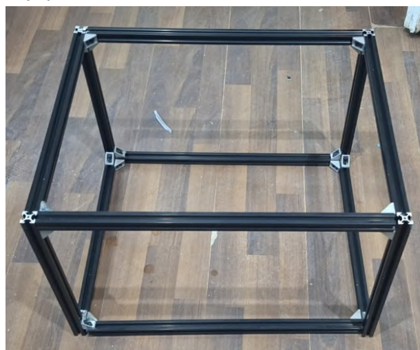
Figure 11: Physical assembly of Leviathon's modular aluminum extrusion frame.
