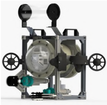
Figure 6: SolidWorks CAD render of Kratos, our previous ROV model.
