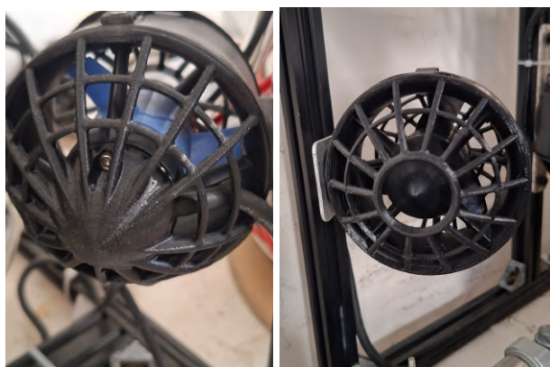
Figure 28: our 3d-printed thruster guards.
