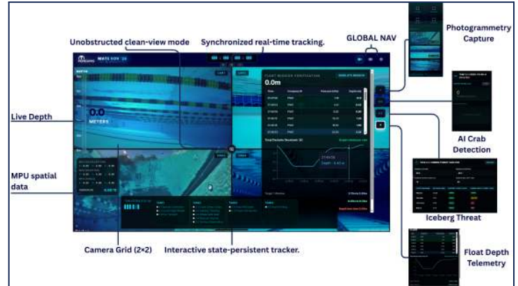
Figure (11): Top Side GUI Task Integration
