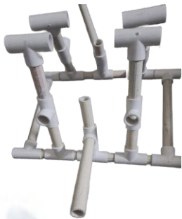
initial assembly of the PVC frame, showcasing the basic cube-like geometry and internal ballast compartments.
