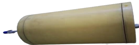
Custom-lathed HDPE electronics enclosure before final assembly and sealing.
