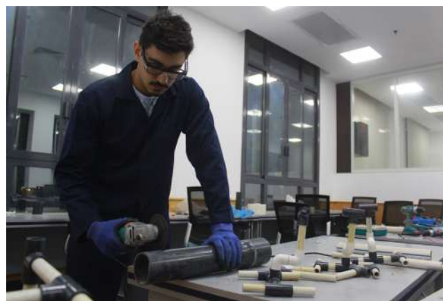
Figure 29: Cutting the PVC pipes for the training track assembly.
