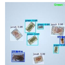
Figure 39: YOLOv8 detection of Green crab samples
