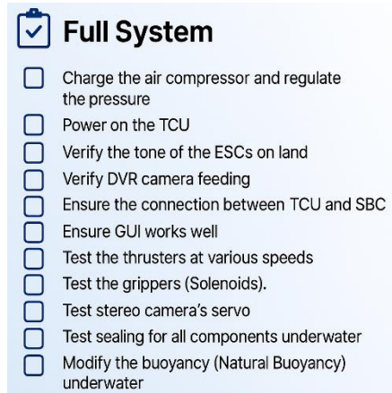
Figure 47: Full System Test
