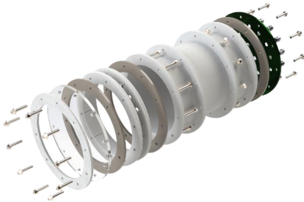
Figure 2-6 Electrical Enclosure Exploded view
