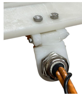
(b) Real Life Photo of NEMESIS's Strain Relief
